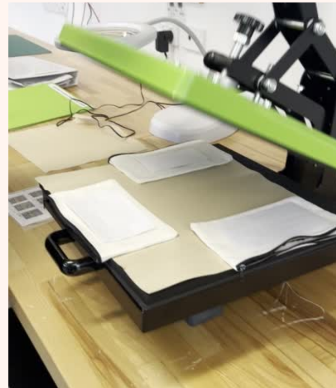
Heat dyeing with sublimation printer
